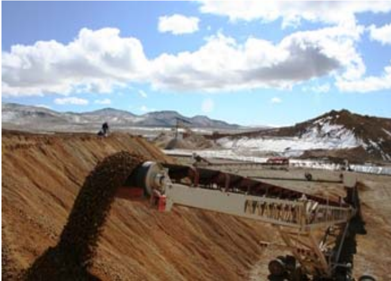
Ore is continually being stacked on the new heap leach pad
