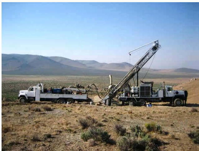
Hoisting the mast of the Schramm Honorine Gold
