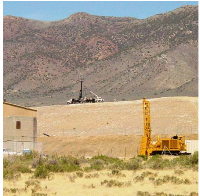
Firstgold Corp.'s reverse circulation drill rig and Sonic Drill on site together.
