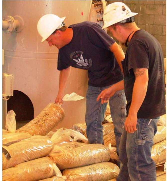
Driller Steve Loughry and associate examine samples taken from heaps via Sonic Drilling.
